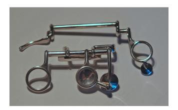
A relatively stable development of this Oehler mechanism can be found on Graessel clarinets. Here, the connection of the high-Emechanism is created by an "eight". The advantages are obvious: stable connection without screw, therefore a thinner axle can be used and the already existing flaps can easily be stored on bushes. So it is also possible to convert a conventionally built Oehler mechanism.
