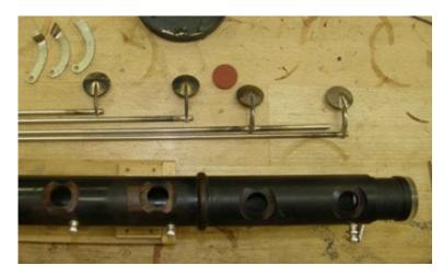
Now the old tone holes (E and Eb) as well as the old post drillings were closed. Then a grenadilla connection piece was made and set and the four new holes drilled to the correct acoustic position. We made the double posts from solid silver and gave the keys a new shape.
